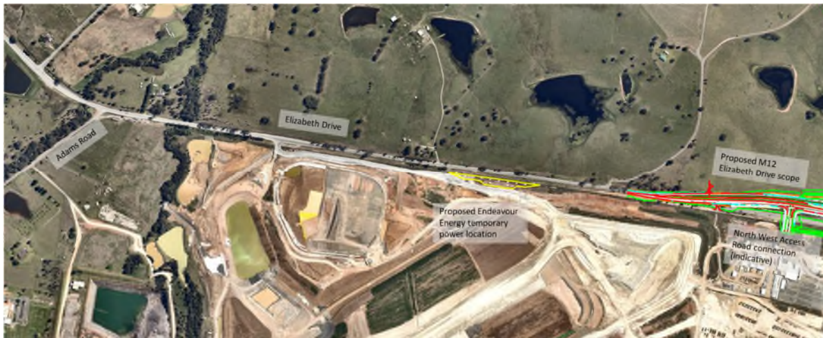
Figure 10: Temporary power supply works on WSA land
