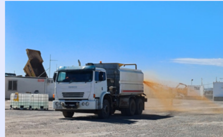
Figure 43 - Dustex application to reduce dust generation on trafficable roads
